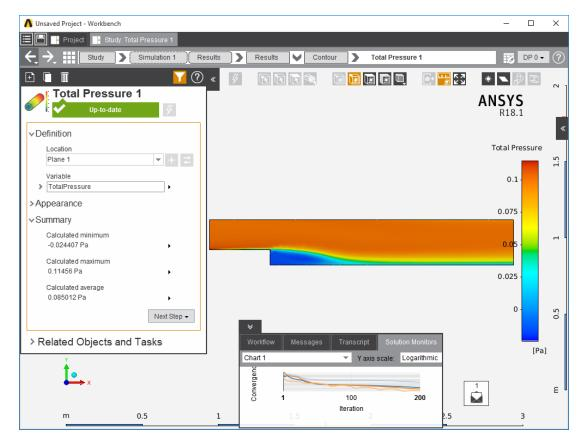
The same thing can be done to plot the velocity field as a contour. Repeat the steps above to create the **Contour**, but make the variable **Velocity Magnitude** instead of **Total Pressure**.
