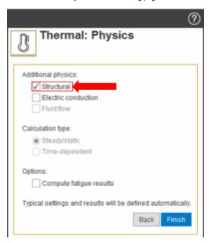
You will be prompted by the **Thermal** template to either **Define new geometry**, **Import geometry file**, or **Connect to active CAD session**. Select **Define new geometry** and press **Next**. For this problem, we will be using the **Steady/static** calculation type and adding **Structural** as an additional physic. Select them in the menu and press **Finish**. The Model Editor will launch automatically.
