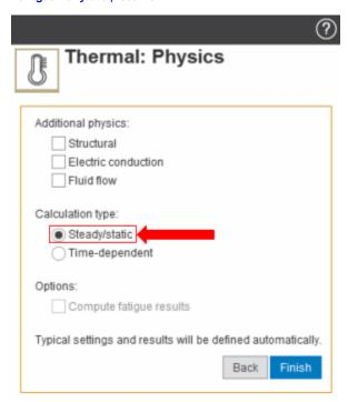
For this problem, we will be using the default **Steady/static** calculation type. Press **Finish**. No additional physics are necessary.
