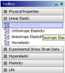
Now, the properties of "Cornellian" need to be entered. Set the Young's Modulus to 2.8e10 Pascals and set Poisson's Ratio to 0.4. Note that the stiffness matrix for the beam element is independent of the Poisson's Ratio. Hence the solution will not change if a different Poisson's Ratio is used.
