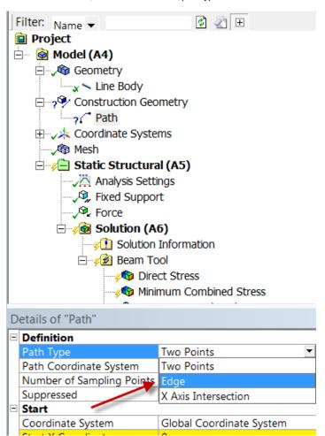
Next, using the Edge Selection filter select the line body in the Graphics window. Back in the Details of "Path" window, select Geometry > Apply.
