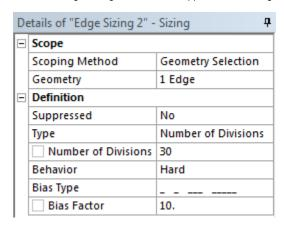
Now we would like to apply an edge sizing to the outlet, the right end of the pipe. Once again, we'll use 30 divisions, with a bias factor of 10 and with the smaller divisions at the top, near the wall. This time, when selecting **Bias Type**, choose the first option, --- - -. This will put the smallest divisions at the top. Other than this, the procedure is the same as for the inlet. When complete, your Details of "Edge Sizing 3" should look like this:
