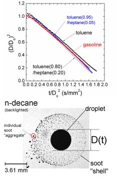
photograph of a n-decane droplet at one evolution of droplet diameter (D); instant during its burning history. slope is the "burning rate"
