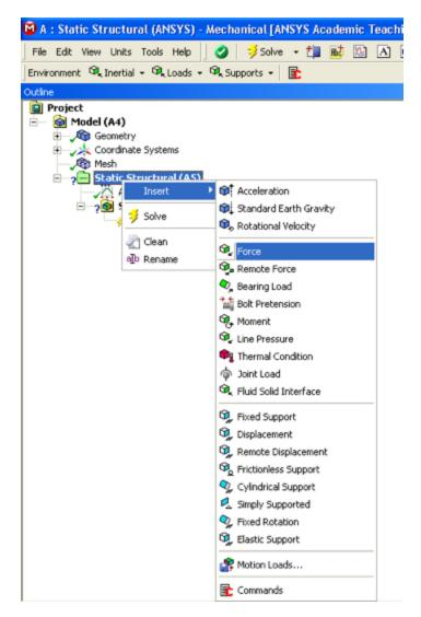
At this point, there should be a *Details of "Force"* window in the lower left corner of the Setup window. Expand *Definition* if it is not already expanded and then change *Define by* to *Components* as seen below.
