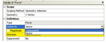
Now, click on the box to the right of Y Component without clicking the Y component button and change the force to -8000N. That is, you should NOT check the box to the left of Y Component. Your *Details of "Force"* window should now look very similar to the following image.
