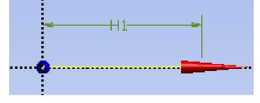
In the *Details View* column a yellow box to the right of *Base Objects* should be highlighted in yellow. Click on the yellow box and then click *apply*. Then, click on the *Generate* button **Generate** button; it is located on the top left portion of the Design Modeler.
