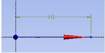
Now, the length of the line will be manually edited. Underneath the *Sketching Toolboxes* there will be a column called *Details View*. In *Details View* there is a subcategory called *Dimensions: 1*. Change the numerical value of H1 to 4 meters and press enter.
