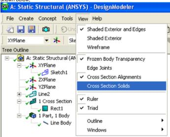
If you click on the *1 Cross Section*, in the *Tree Outline* and then click on the light blue dot, a three dimensionally rendered beam in an isometric view. Note that this is merely a visualization; our beam model is only a line.
