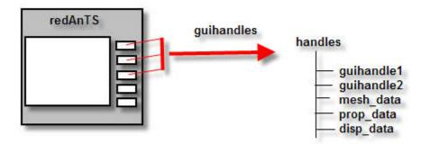
In the above figure, the fields *guihandle1* and *guihandle2* are handles for "objects" in the *redAnTS* GUI. The field *mesh\_data* contains the mesh information (the x and y coordinates of the nodes etc.) and is, in turn, a structure. The field *prop\_data* contains the material properties (E, nu) and is also a structure. Yada yada yada.
