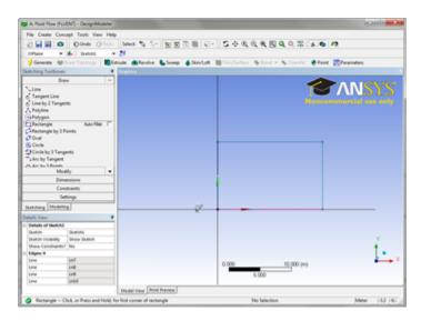
Because the wall has two sections, an isothermal section and a heated section, we will need to split the upper edge. To split the edge, select the *Modify* ta b in the *Sketching Toolboxes* window, and select Split . Next, click any point along the upper surface of the rectangle. This will split the line into 2 segments.
