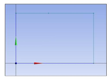
It turns out that to get a nice regular mesh, the bottom edge should also be split in the same way. So split the bottom edge as well (don't worry about the location, we'll adjust that next).
