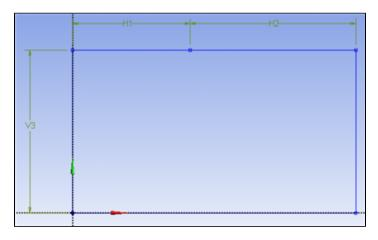
We can set the dimension in the *Details View* window. In the *Details View* window, change *H1* to 5.76, *H2* to 2.88, and *V3* to .06. You can zoom in/out using the middle mouse wheel. You can move the dimensions by selecting *Dimensions* > *Move* and then dragging the labels by grabbing them with the mouse.
