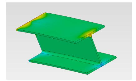
The Euler-Bernoulli theory predicts normal stresses in the absence of out=of=plane stresses (which are presumed negligibly small. Here the out-of-plane ZZ component of stress is predicted to be approximately 810 psi, i.e on the order of normal stresses due to bending alone. These substantial out-of-plane stresses result in Poisson effects on the normal wall stress, increasing its value substantially.
