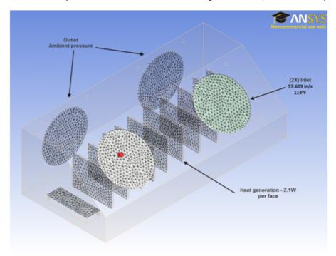
The box itself is ABS plastic, the components will be modeled as copper, and the material properties are shown in the table below.
