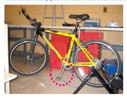
Material properties: The bicycle crank's material is aluminum 6061-t6. The Young's modulus is 10,000 ksi, and the Poisson's Ratio is .33.
