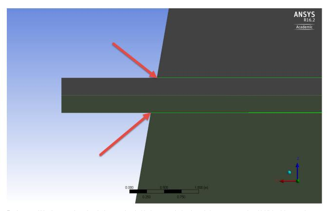
For the second blend, you need to select the bottom edges inside the groove. In the picture below you can see them highlighted, but note that to ease the understanding, a "sliced" geometry is shown. Your geometry will look like this by the end of the above video!
