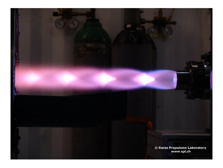
For that, we need to design a Nozzle that has a measured exit pressure **smaller** than the ambient pressure. This means that the nozzle is "too big" and will end up expanding the flow too much.
