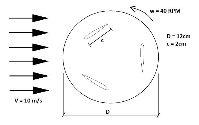
Consider an uniform flow of V = 10m/s passing through a Vertical Axis Wind Turbine (VAWT) as sketched above. The VAWT has a diameter of 12cm and 3 equally spaced blades, each one with a chord length of 2cm. For simplification, consider that it spins with a constant angular velocity of 40 RPM\*. The center of each blade is located 0.04m from the center of the hub.
