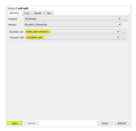
Next, insert a chart (Insert > Chart). Name it "Veloc at blade". Under "Data Series" tab, change the Location to the created "wall right".
