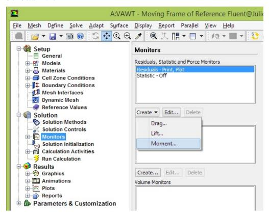
Under "Options", check the boxes to "Print to Console" and "Plot". Under "Wall Zones", select "wall\_blade\_right". Change the "Moment Center" to X=0.04m and Y=0. Click Ok.
