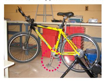
$\textbf{Material properties} : The \ bicycle \ crank's \ material \ is \ aluminum \ 6061-t6. \ The \ Young's \ modulus \ is \ \underline{10,000 \ ksi}, \ and \ the \ Poisson's \ Ratio \ is \ \underline{0.33} \ .$
