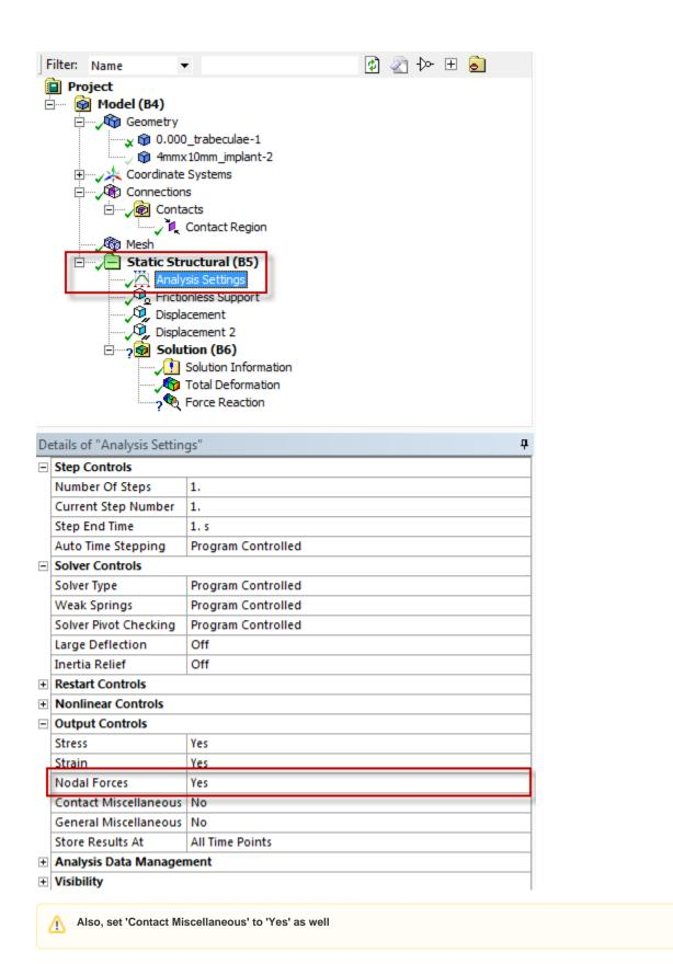
Then you must RE-SOLVE THE SOLUTION, or the new output control that you included will not be taken into effect. To do this, delete the probe and then rerun. Once complete, you may re-insert the reaction probe and select Contact, and you will no longer get an error from Output Controls.
