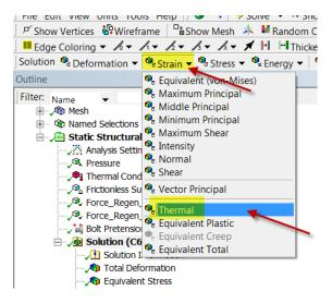
Check that the thermal strain reported by ANSYS for all parts compares well with the expected value from alpha\*(dT).
