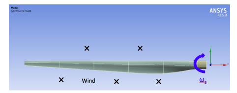
The turbulent wind is flows towards the negative z-direction (into the page on the above diagram) at 12 m/s which is a typical rated wind speed for a turbine this size. This incoming flow makes the blade rotate at an angular velocity of -2.22 rad/s about the z-axis (the blade is thus spinning clockwise when looking at it from the front, like most real wind turbines). Note that to represent the blade being connected to a hub, the blade root is offset from the axis of rotation by 1 meter.
