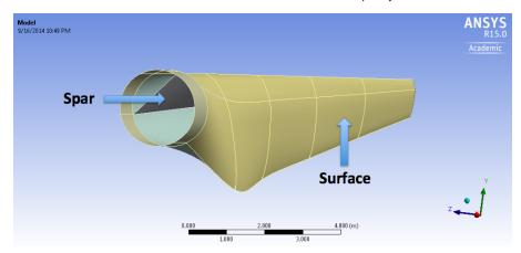
The blade is composed of an outer surface and an inner spar. The thickness of the outside surface linearly decreases from 0.1 m at the root to 0.005 m at the tip. The spar has a similar thickness behavior with 0.1 m at its closest point to the root and 0.03 m at the tip. To sum up, here are the thickness specifications needed along with their location with respect to the global coordinate system (which represents the center of an imaginary hub and thus the center of rotation).
