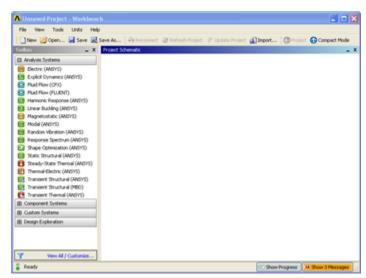
To begin, we need to tell ANSYS what kind of simulation we are doing. If you look to the left of the start up window, you will see the Toolbox Window. Take a look through the different selections. The plate with a hole is a static structural simulation. Load the static structural tool box by dragging and dropping it into the Project Schematic.
