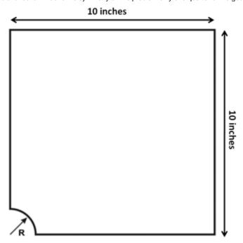
The radius of the hole is the design variable. Furthermore, the radius is constrained between a minimum value of 1.0 inch and a maximum value of 2.5
