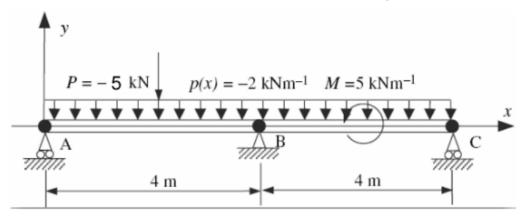
Consider a two-span beam shown above. The beam is subjected to uniformly distributed loading, point force at x=2m and moment at x=6m about the Z-axis, as shown. The beam bending stiffness is El=2 x 10^7 Nm^2.
