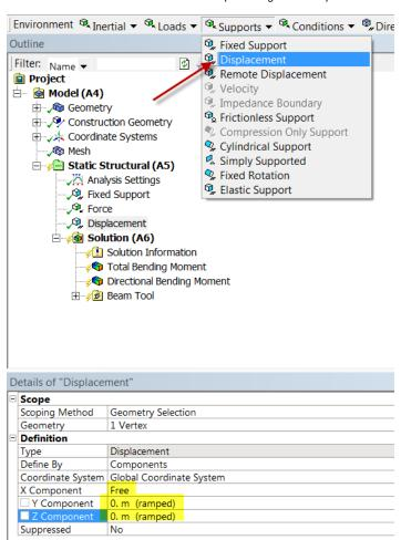
5. You also need to add a constraint at one vertex to prevent rotation about the x axis as discussed in the truss tutorial in our free online ANSYS course at edx.org. This can be done by selecting Supports > Fixed Rotation as shown below.
