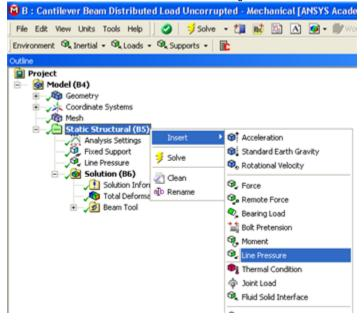
You will then need to apply the line pressure to the line, specify the magnitude and direction of the line pressure and lastly have ANSYS solve the system.
