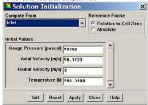
Click *Init*. The above values of pressure, velocity and temperature are now assigned to each cell in the grid. This completes the initialization. *Close* the window.
