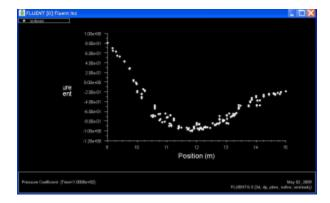
We see that there is a lot of scatter in our data, so we will be creating a line along the sphere to try and get a better picture of the pressure coefficient. To accomplish this we will create a surface of Z-axis position zero, and plot the line  $y^2+(x-12)^2-9$ , which is the equation of a ring around the sphere in the x-y plane.
