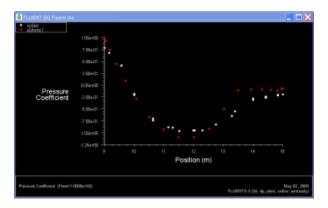
The Red dots are the experimental data (labeled "sphere1"), while the white dots are our data (labeled CPline).
