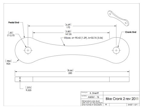
We also know that "P" is 100 lbs and "E" is 10,000 ksi. The tricky part is to determine the moment of inertia. Recall that for a rectangular cross-section of height h and depth b,
