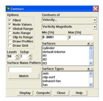
Under Contours of, choose Velocity.. and Vorticity Magnitude. Disable Auto Range and Clip to Range from the Options group box. Enter 0.0001 and 2 for Min and Max, respectively. Select Levels to 50. Click Display.
