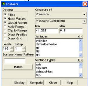
Under *Contours of*, choose *Pressure..* and *Pressure Coefficient*. Select the *Filled* option. Increase the number of contour levels plotted. Set *Levels* to 1 00. Disable *Auto Range* and *Clip to Range* from the *Options* group box. Enter -1.225 and 0.5 for *Min* and *Max*, respectively. Click *Display*.
