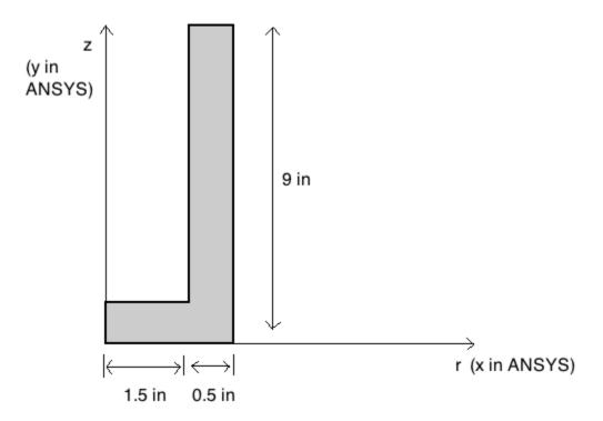
We use symmetry to model only half the total length of the cylinder.
