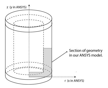
In ANSYS, the radial direction is x (rather than r) and the axial direction is y (rather than z). Confusing! We recommend that in an axisymmetric analysis, you think of the directions in ANSYS as radial & axial rather than "x" and "y".
