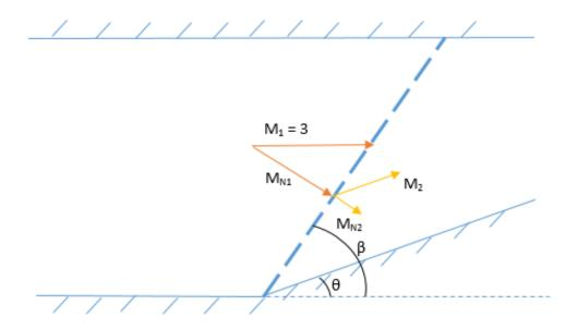
Step 1: We then look at the Theta-Beta-M chart here we can find what the shock angle is corresponding to our conditions. The line M = 3 with wedge angle theta at 15 degrees corresponds to a shock angle beta of about 32 degrees.
