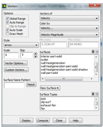
Make sure the settings of the menu match the figure above: namely *Vectors of > Velocity*, *Color by > Velocity*, and set the second box as *Velocity Magnitude*. To see the velocity vectors, press *Display*.
