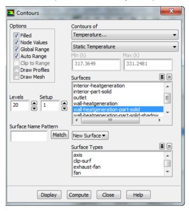
Once these parameters are set, press *Display* to see the temperature contours.
