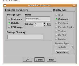
For **Window**, we use number 3, which means that the velocity magnitude window is being recorded (You need to choose proper window number if you have different windows); then click **Set** and the figure window 3 will show up. Under **Display Type**, choose **Contours**:
