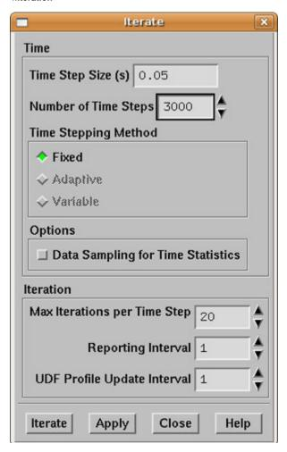
Because the flow is unsteady, we need to define the size of the time step. In this case we use 0.05s as the time step and run the simulation for 3000 time steps. Note that in terms of the dimensionless scale, the time step is 5% of the residence time (d/U).
