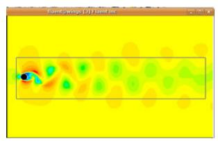
This window will record the velocity contours every a few time steps as specified while the flow is evolving.
