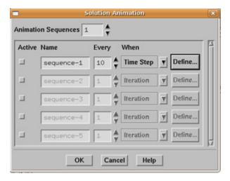
Choose **Time Step** under **When**. Type 10 (or up to 50) in **Every** box so that a frame is recorded every 10 time steps. Note that the more frequently you record a frame, the larger data the code will produce. You may delete the data files generated by Fluent after creating the animation (sequence.xxx.hmf). Click **Define...**
