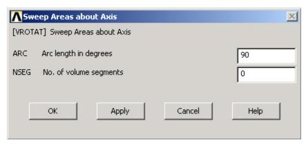
Repeat the same procedure to generate the lower volume. Start by selecting the lower area (2). Click *OK*. Then select keypoint 3 first and then keypoint 4, click *OK*. In the following menu, enter 90 for *ARC Arc length in degrees* and 0 for *NSEG No. of volume segments*. Click *OK*.
