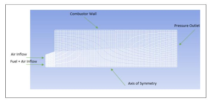
This is a partially premixed combustion case, which has inflows that reflect both premixed (fuel inflow) and nonpremixed (fuel and air mixing) conditions.
