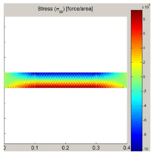
We expect a pure bending stress in the central region between the two applied forces. The stress is tensile on the bottom surface and compressive on the top surface as expected. Elementary beam theory predicts the bending stress as  $_{xx} = My/I$ . Here
