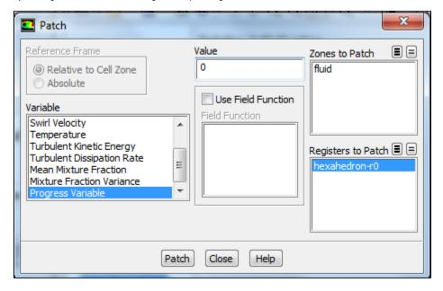
Now go back to Solution Controls and click "Equations". Reselect the PDF and Premixed Combustion options so that all options are highlighted and will be solved for. Press OK. In Solution Methods, make sure that all solvers (Momentum, Swirl Velocity, and Turbulent Kinetic Energy) are set to a second order solver scheme.
