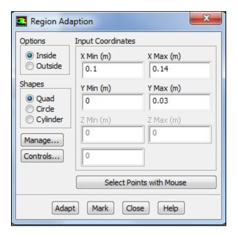
Patch this region by going to Solution Initialization, and click "Patch". Select "Progress Variable" as the variable, and patch the region that you just marked by clicking "Patch". Close the dialogue after patching.
