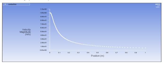
You can see that the axial velocity at the centerline (U\_center) decreases sharply after the inlet, and that it will asymptotically approach 0m/s far from the jet. However, the half-width (Y distance at which U=U\_center/2) increases along X as the spray expands.
