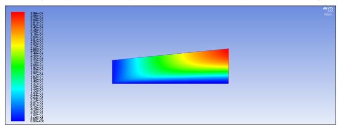
From these contours, you can observe that the air is being entrained near the jet inlet, and that the jet expands slightly along the x-direction. By knowing that the flow velocity is related to the stream function by U = /y and V = -/x, one can see that the stream function values will be smaller in the entrainment and jet stream areas, because the flow is more strongly linear there.
