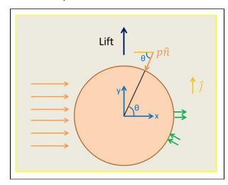
Consider the case of a fluid flowing past a cylinder, as in the steady cylinder case, with a Reynolds number of 20.
