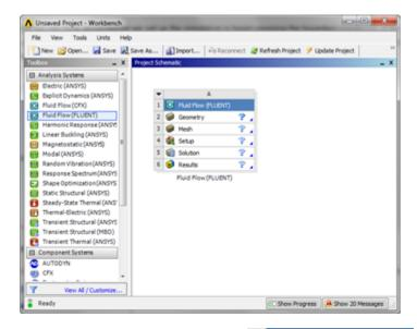
Right click the top box of the project schematic ready to create the geometry for the simulation.
