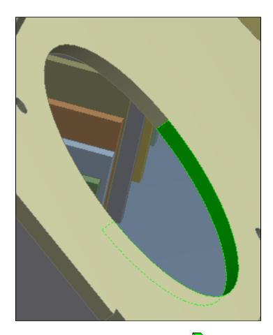
To select these surfaces, use the *Face Selection Filter* Hold down CTRL to select multiple surfaces at once. When all the surfaces have been selected, press *Faces > Apply* in the *Details* window. 40 surfaces should have been selected.
