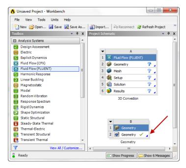
This will open the *Design Modeler*. When the design modeler loads, we will first need to specify a standard unit. Select *Inch* and press *OK*.
