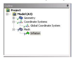
The parameters for the *Inflation* are given in the *Details Pane*. With *Geometry* highlighted, select the cylinder using body selection tool, click *Apply*.
