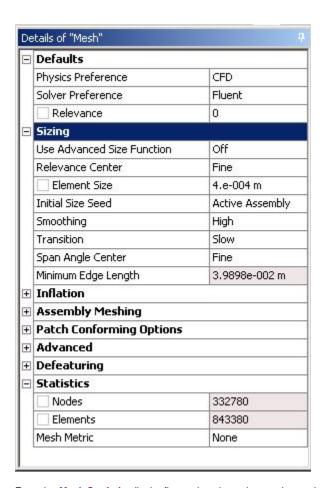
From the *Mesh Statistics* (in the figure above) we observe that we have about 0.85 million elements which would require multiple cores to run the simulation.
