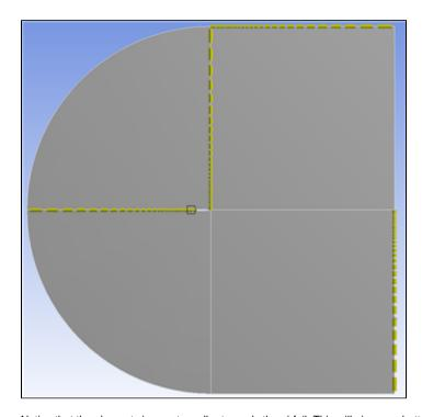
Notice that the element sizes get smaller towards the airfoil. This will give us a better resolution around the airfoil where the flow gets more complicated. Create a new edge sizing with the same parameters, but choose the 4 remaining straight edges (see figure below). The number of divisions will still be 50, but now will be selecting a different biasing type by selecting the second Bias option: Bias > - - - ------. Again, set the Bias Factor to 150
