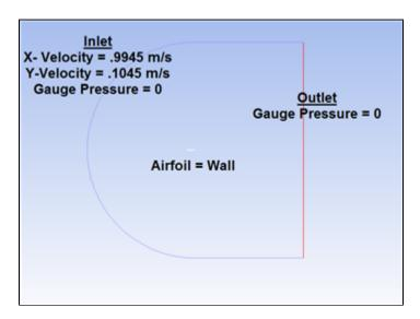
The edges highlighted blue are the inlet, the edges highlighted red are the outlet, and the airfoil is highlighted white in the middle. Now we are ready to
