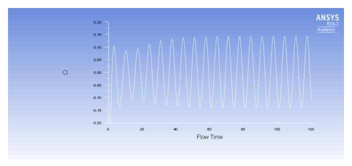
Above, we see the variation of the lift coefficient with the folw time with the region patch. This patch was using .5 < x < 32 and 0 < y < 32. Note how we see the shedding more quickly than if we had not patched the region.
