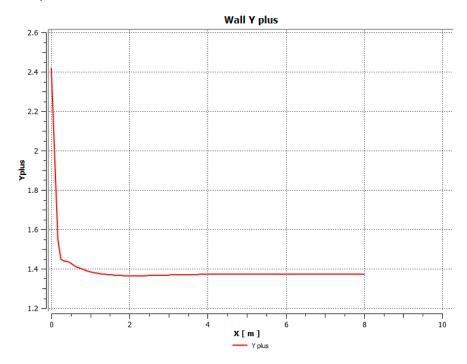
As we can see, the wall \_y+\_value is between roughly 1.35 and 2.45. Since this is less than 5, the near-wall grid resolution is acceptable.
