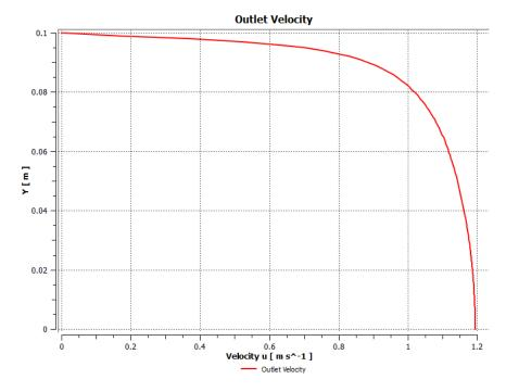
The axial velocity is maximum at the centerline and zero at the wall to satisfy the no-slip boundary condition for viscous flow. Compare qualitatively the near-wall velocity gradient normal to the wall with the laminar case. Which is larger? From this, what can you say about the relative strengths of near-wall mixing in the laminar and turbulent cases?
