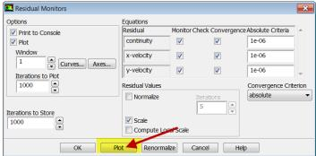
It looks like my solution hasn't converged, so I need to run more iterations by selecting *Run Calculation*. You may want to increase the number of iterations to, say, 1000. Ensure that you have a converged solution and save the project.
