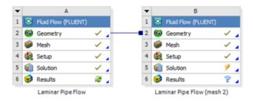
Next, double click on the *Mesh* cell of the *Laminar Pipe Flow (mesh 2)* project. A new ANSYS Mesher window will open. Under *Outline*, expand *Mesh* and click on *Edge Sizing*, as shown below.
