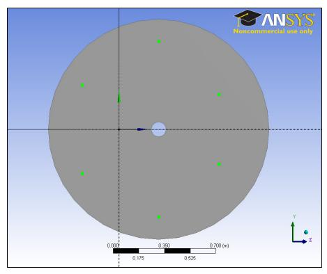
Now that the guiding points are created, we need to create a sketch for the diameter of the truss line bodies. First, we need to create a plane that the sketch is based upon: it needs to be the same plane as the top of the circular base support.
