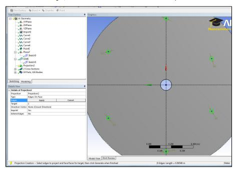
Generate the Projection. This now has created lines on the Circular Mount Pad. We can now use the created surface area as a connection surface for the Setup step.
