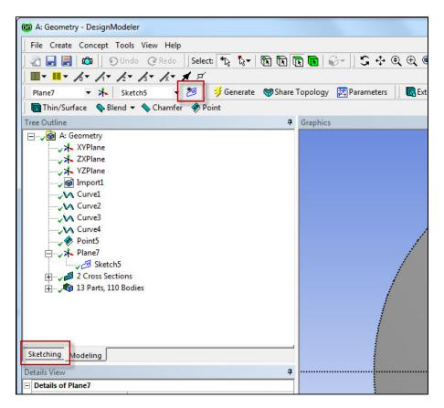
Create a circle of .03m diameter centered around the construction points. There are a total of six circles on this sketch.
