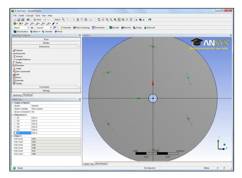
Return to the modelling tab. Now that the sketch has been created, we actually have to apply it to the geometry. Otherwise, it is just an unattached sketch. Since we are just making a surface area to attach a connection to, all we need to do is project some lines into the surface. This requires two steps: 1. Create a Concept > Lines from Sketchs. Select the sketch you created, and Add Frozen.
