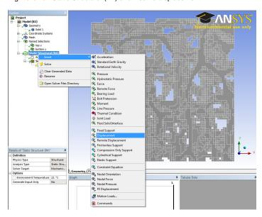
Change the Scoping Method to *Named Selection* and select *top y*. Enter *-0.5 mm* for the *Y Component*. This will assign a 0.5 mm displacement to the model in the -y direction on the faces selected for *top y*.
