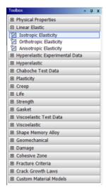
In the properties window, expand Isotropic Elasticity and enter 1e9 Pa for Young's Modulus and 0.3 for Poisson's Ratio.
