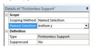
This will constraint the displacement in the y direction but the model is allowed to displace in the x direction. This is very similar to the conditions of a roller support.
