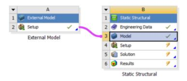
We have not defined the material for this model so we will do that before we proceed. Double click on *Engineering Data*. Click on "click here to add a new material" to create a new material. Name the new material "Bone". Expand *Linear Elastic* and double click on *Isotropic Elasticity*.
