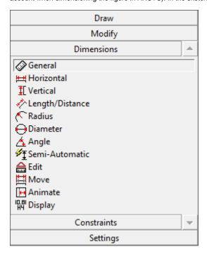
This tool will allow you to define dimensions that you can specify. We need to specify the rectangle's length and width, and the circle's radius. Use the tool to define the height of the rectangle (the right edge of the geometry), the length of the rectangle (the top edge of the rectangle), and the radius of the circle. You should end up with the following window.
