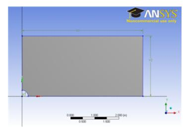
Close the Deign Modeler (don't worry, the geometry will be saved in the project automatically). Now we are ready to mesh the geometry.
